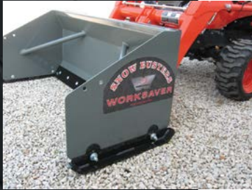
End plates with gentle slope design
